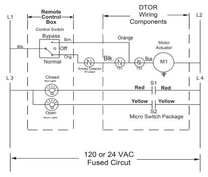
**Note:** Wires indicated are for M/S Package mounted on the right hand side of the damper. If the M/S package is on the left hand side, then the open/close wires will need to be switched.
