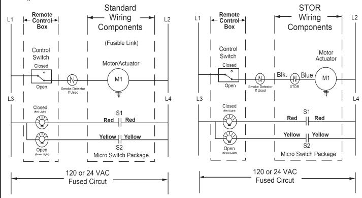
Note: Boxes are standardly shipped with 120vac lights. Special and indicate on order 24vac or vdc lights if needed.
